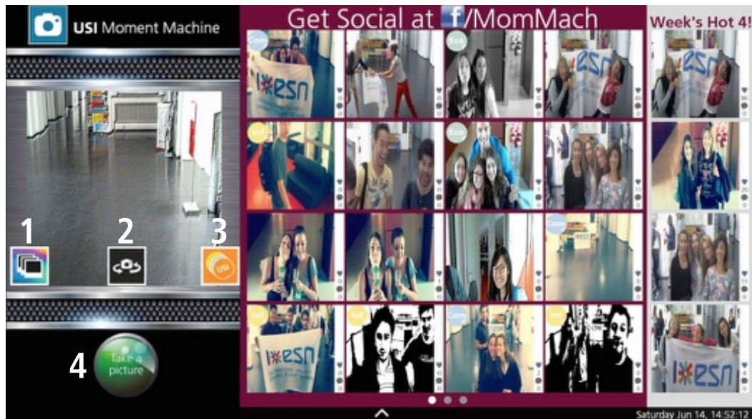
(a) Moment Machine 2.0 user interface: 1) button for changing the filters, 2) button to mirror the image, 3) button for stickers, and 4) button to take the photos.
